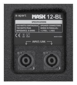
Input: the signal from a power amplifier must be connected to the input/link speakon<sup>®</sup> connector. The connectors are equivalent and internally wired in parallel. Connector 1+ (positive) and 1- (negative) are used. 2+ and 2- are not connected.
