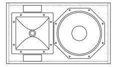
rotate HF horn 90° for horizontal orientation
