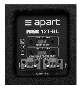
Input: the signal from a power amplifier must be connected to the input/link euroblock connector. The connectors are equivalent and internally wired in parallel.
