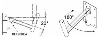
For your safety, we strongly advise to secure the speaker using a safety chain. The chain and the necessary mounting hardware(eyebolts) are not supplied with this bracket. The chain and the attachment eyebolts should be capable of supporting at least 12 times the weight of the speaker. Mount the safety chain in such a way that the speaker or the supporting hardware won't drop more than 20 cm.
