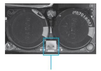
110 VAC operation: it is possible to operate the unit at 110 (115) VAC.
