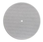
The Apart CM608D is a 2-way 8 ohm built-in design ceiling loudspeaker. The loudspeaker has a 6 ½" woofer and a 1" coaxial tweeter. CM608D is the perfect choice for the distribution of microphone calls and background music. The mounting frame is made of high quality ABS. The steel grille is kept in place by strong magnets.
