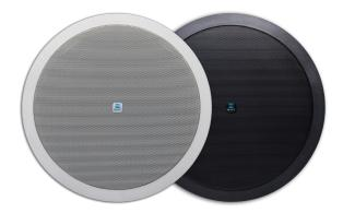
The Apart CMX20T is a 2-way 100V/70V/16 ohm built-in ceiling loudspeaker. The loudspeaker has a 8" woofer, a 1" coaxial tweeter and a high quality 100/70 volt speaker line transformer with multiple power taps. CMX20T is the perfect choice for the distribution of microphone calls and background music. The mounting frame is made of high quality ABS. CMX20T is available in black and white.
